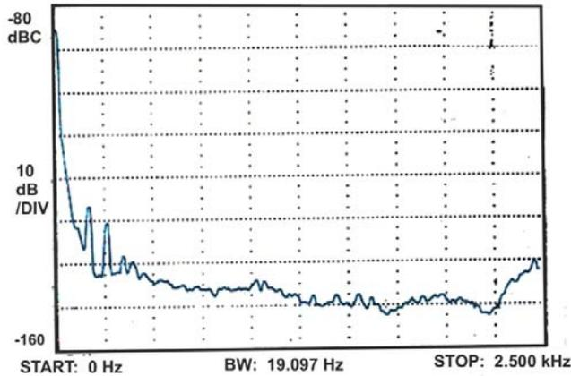
Fig. 7. Mechanical resonance for the 0.006" Kovar lead-frame (new QRM).
