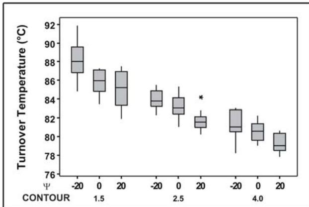
Fig. 11. Turnover temperature results grouped by contour and  $\Psi$  angle.
