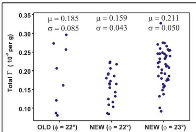
Fig. 8. Typical g-sensitivity results for the old and new QRM resonators.
