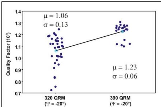
Fig. 15. 390 QRM Q-factor ( $\phi = 23^\circ$  and  $\Psi = -20^\circ$ ).
