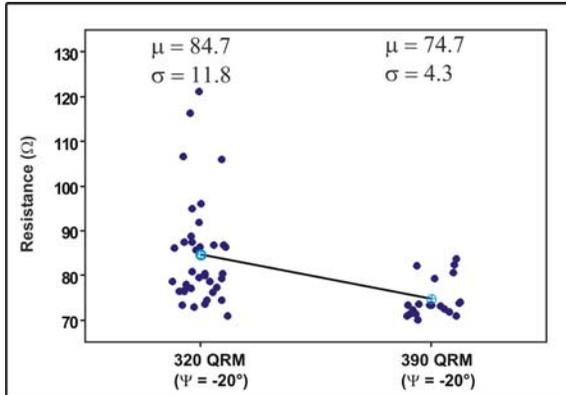
Fig. 14. 390 QRM resistance ( $\phi = 23^\circ$  and  $\Psi = -20^\circ$ ).
