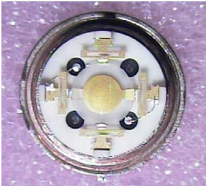
Fig. 2. Old 8mm (0.315") QRM resonator structure.
