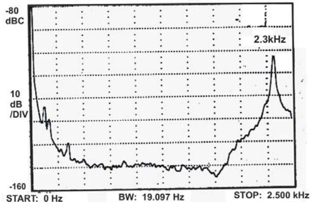
Fig. 6. Mechanical resonance for the 0.004" Kovar lead-frame (new QRM).
