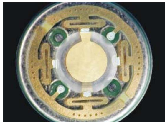
Fig. 9. 320 4F QRM resonator structure.
