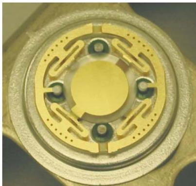
Fig. 3. New 0.320" QRM resonator structure.
