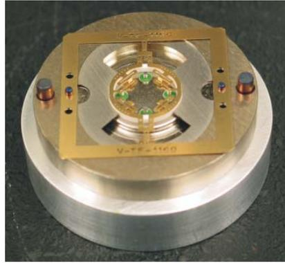
Fig. 5. Kovar assembly fixture (alignment of the lead-frame).
