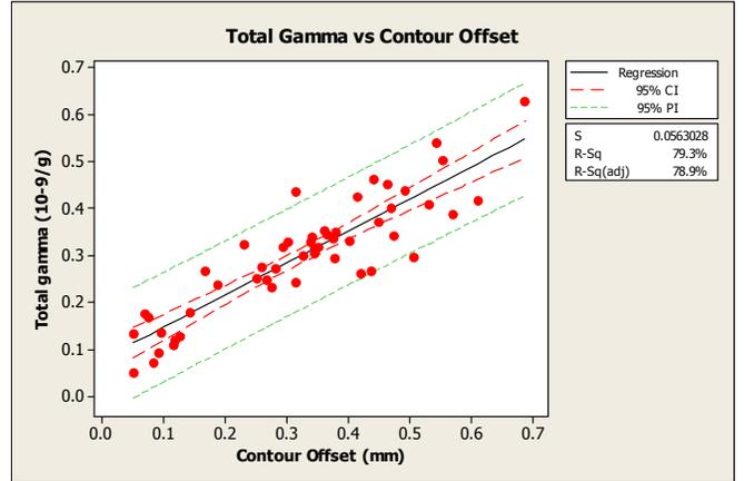
Fig 8 g-sensitivity versus contour offset for measured group
