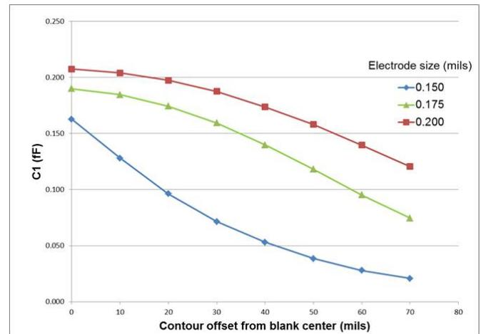
Fig 4  $C1$  vs. contour offset for various electrode diameters
