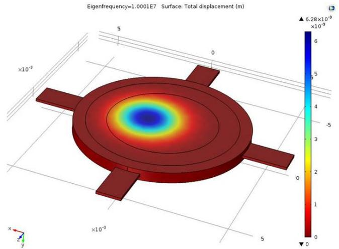
Fig 3 Contour map of resonator with offset contour
