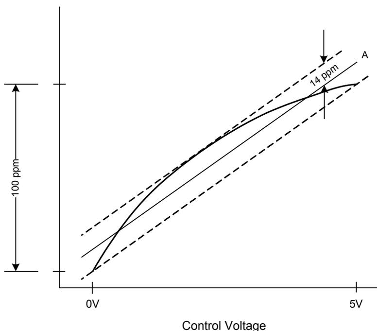
The VCXO which produces the characteristic indicated in Figure 2 uses a hyper-abrupt junction varactor diode, biased to accommodate a bipolar ( $\pm$ ) control voltage. The VCXO which produces the characteristic in Figure 3 uses an abrupt junction varactor diode with an applied unipolar control voltage (positive in this case).
