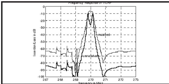
Figure 3. 4-Pole TCRF Design for IF Applications
