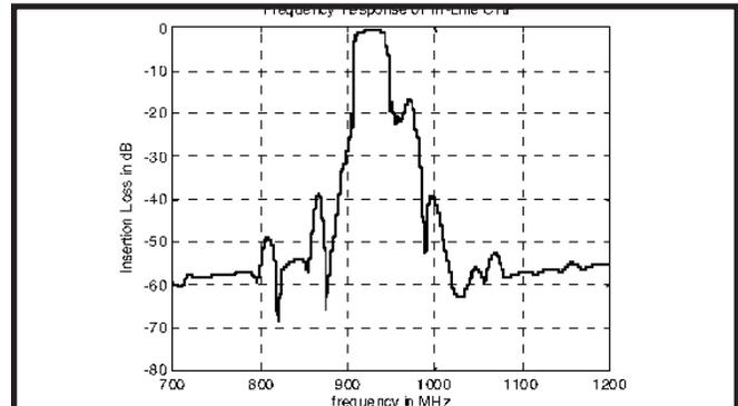
Figure 1. In-line CRF Design for RF Applications
